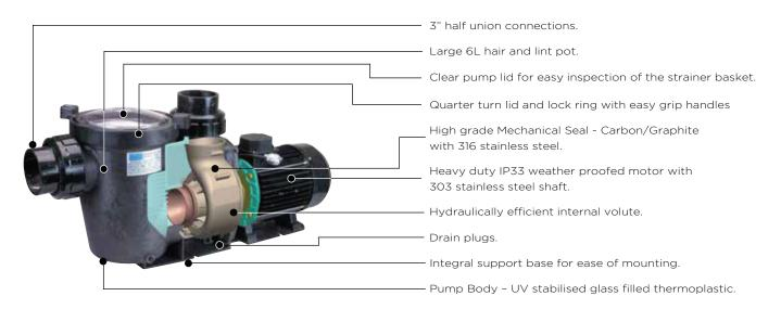
The Ecostar Plus has been designed to provide a substantially quieter operation with even higher flow rates and higher head than the previous Ecostar models. Ecostar Plus has improved the hydraulic efficiency of the pump with the introduction of an internal volute. The volute's hydraulic design provides a natural balanced water flow and reduces hydraulic turbulence.
